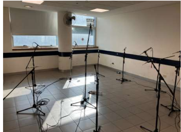
(d) Microphone layout surrounding the machine under test, another perspective.
