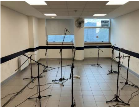
(a) Microphone layout surrounding the machine under test.
